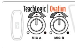
9. **Handheld Mic:** Repeat this process using the MIC B channel to set the ideal volume level. Turn "ON" the handheld mic by tapping the power button once. To enter pairing mode, press and hold the Push to Talk (PTT) button and Power button at the same time for 3 seconds. When in pairing mode, mic will begin to fast blink green. Continue from Step 5 above.
