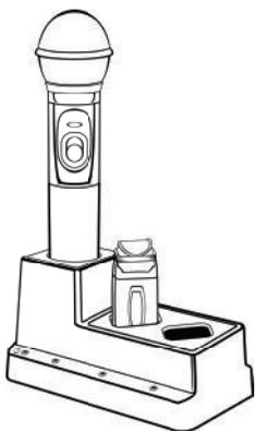
**Do not force mics into the cradle. Ensure that both the charger and Sapphire are aligned in the same direction facing front as shown.**
