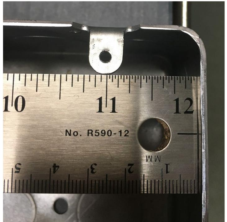
Not okay for fit (below). Observe box too narrow to fit circuit board. See at right edge. The fact that box is 3-gang width, the mounting holes position faceplate and circuit board as shown.
