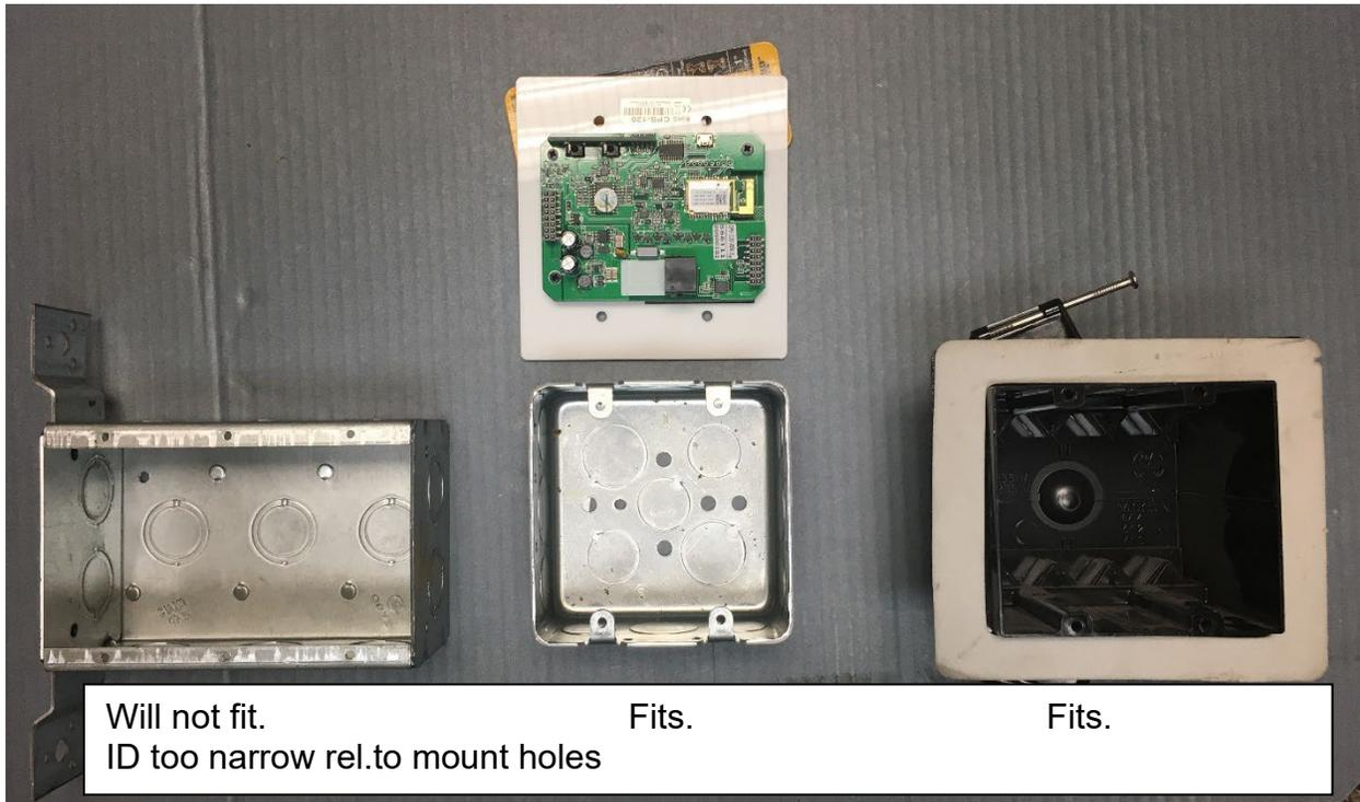
The side clearance from mounting holes in box to inside edge of box must be greater than 24.5mm (31/32 inch). An okay fit is a full 1.00 inch from center of faceplate mounting screw holes to inside edge of box.
