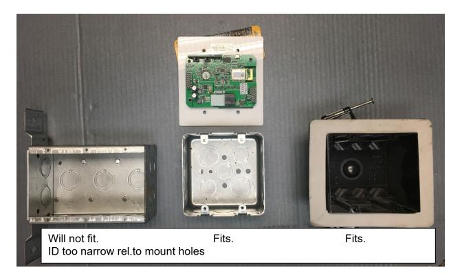
The side clearance from mounting holes in box to inside edge of box must be greater than 24.5mm (31/32 inch). An okay fit is a full 1.00 inch from center of faceplate mounting screw holes to inside edge of box.
